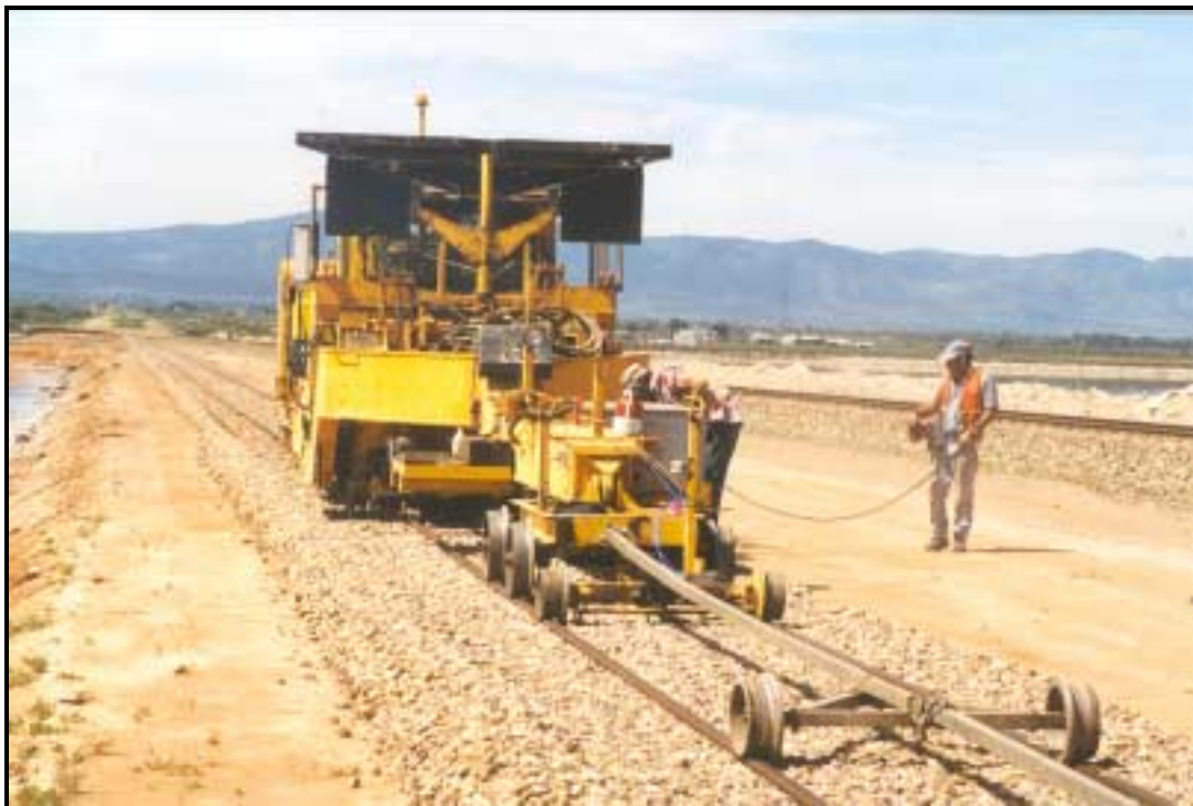
PRR's Mark II Torsion Beam Tamper 'fanging' across Lake Knockout with ex CR Trackman, Kenny White on the 'wander lead'.
